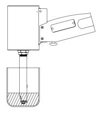
Daily cleaning and lubrication of nose assembly will greatly reduce downtime and increase life of components. Using sewing machine oil, or an equivalent cleaner/lubricant, follow instructions below.
